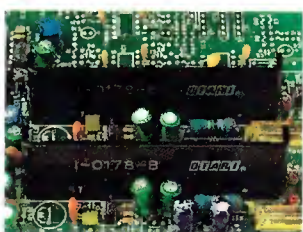
High slew-rate operational amplifiers and premium components contribute to the MTR-15's superb sonic performance.
